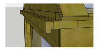
Fine tune your sliding door by installing glides on the top edge. These will allow the door to slide smoothly in the wood channel.
