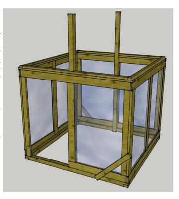
Securely attach center posts by screwing through the front and back middle frames with 3" deck screws.
