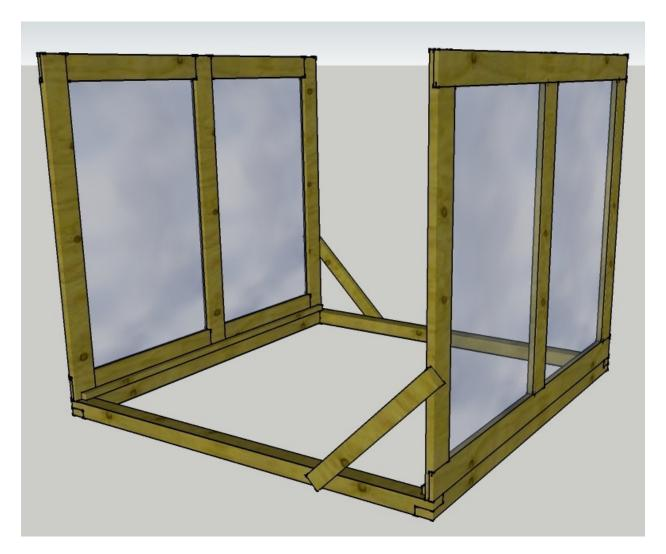
Double check at this point that your internal measurement between the two side walls is 89.5". If it isn't you will need to trim or plane your front and back walls so that they fit.
