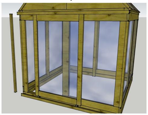
The left stop should be attached to the structure with a 3" deck screw every 6".
