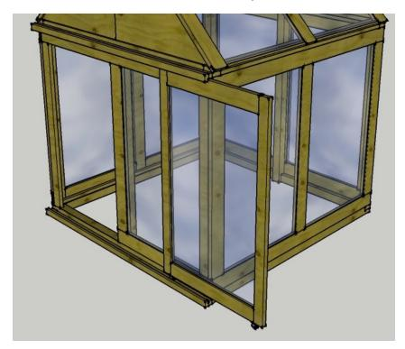
To limit the range of motion to the left is a full length stop. This will not only stop the door from rolling out of the track it will provide a secure face to install a hasp or lock to should you choose.
