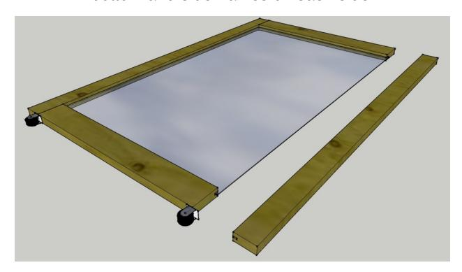
Install the right side of the frame in the same way as the left. Pre drill the holes for your 5" screws. Apply exterior wood glue to the mating wood faces and a thin bead of silicone into the glass slot. Press the right frame into place and once your position is set screw down.
