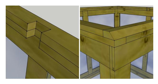
Now you can tilt your center posts into position. The lap you cut into the end of center post will overlap the sill plate at the bottom. The center post will rest in the notches you have prepared in the top plates.
