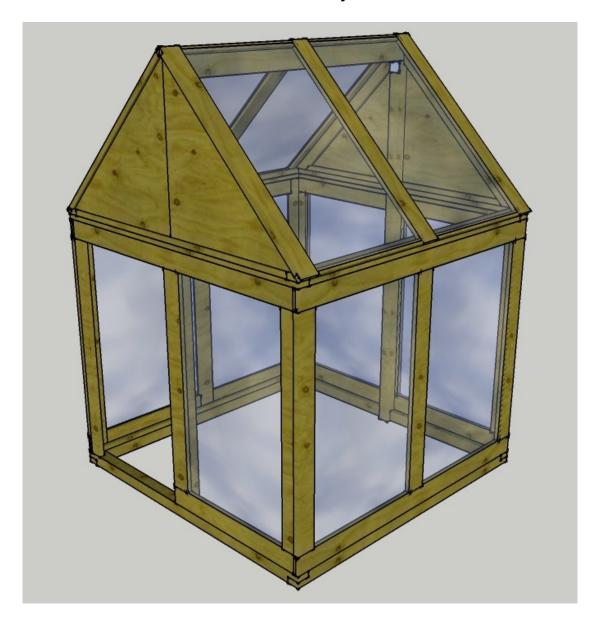
Once the construction adhesive has set on the gable panels the structure is very strong and it is safe to remove the temporary angle braces you installed before.
